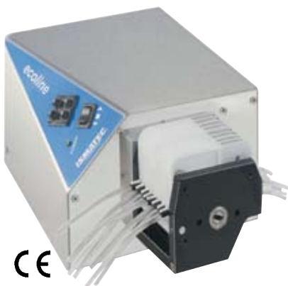
Ecoline VC-MS/CA8-6 0.005–150 ml/min 8 channels 6 rollers
